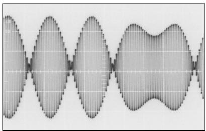
Figure 8.2 – Output RDS signal on oscilloscope (horizontal: 200 µs/div, vertical: 200 mV/div).
