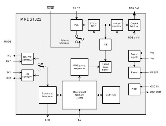
Figure 1.1 – Internal logical structure (simplified)
