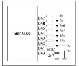
Figure 3.7 – 6 (or 7) -bit D/A converter network.
