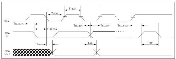
Figure 2.1 – I<sup>2</sup>C bus timing
