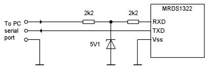
Figure 4.2 – Simple interfacing the MRDS1322 to a PC serial port in mode 1.
