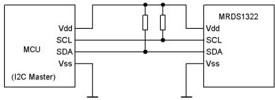
Figure 4.3 – Interfacing the MRDS1322 in mode 3.
