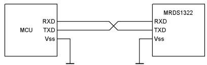
Figure 4.1 – Interfacing the MRDS1322 in mode 0 or 2.
